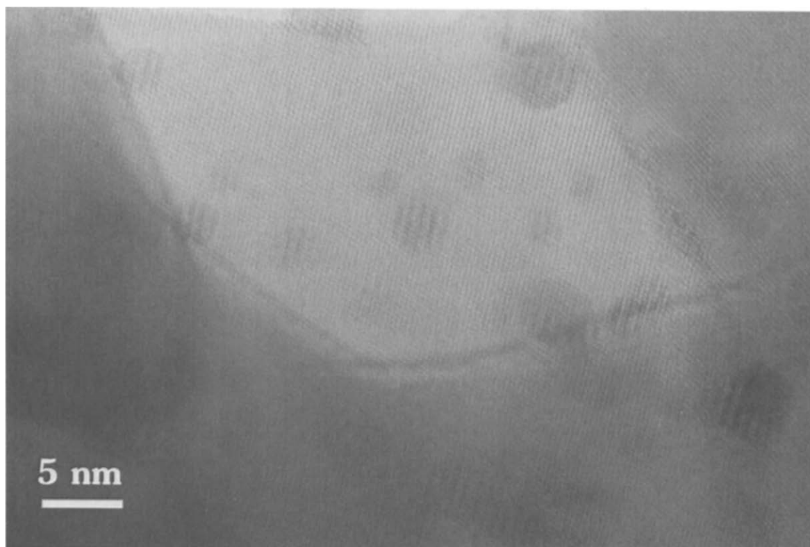
Fig. 10. HREM image for rhodium crystallites in planar projection on ceria. Metal and support [111] axes are in parallel orientation. Zone axis [110] . Sample reduced at 1173 K.
